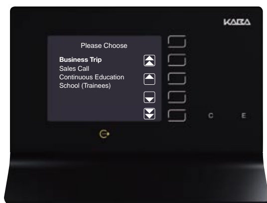
Example work travel - step 3 After a successful entry, a list of reasons for the absence appears. The employee chooses and confirms the choice with "E" (Enter).
